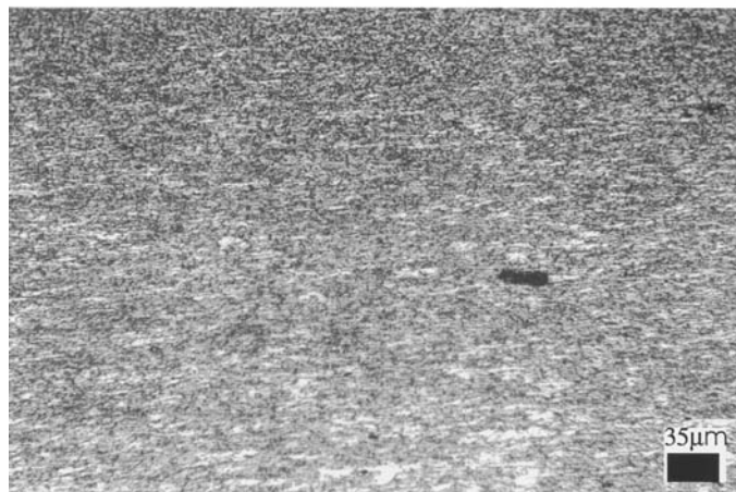
FIG. 17—Local recrystallization seen in an A53 fragment after the detonation of Composition C4.
